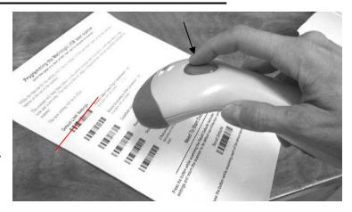
Next, press the button while scanning each of the barcodes below for the default LINK settings. The new LINK settings will be in effect.
